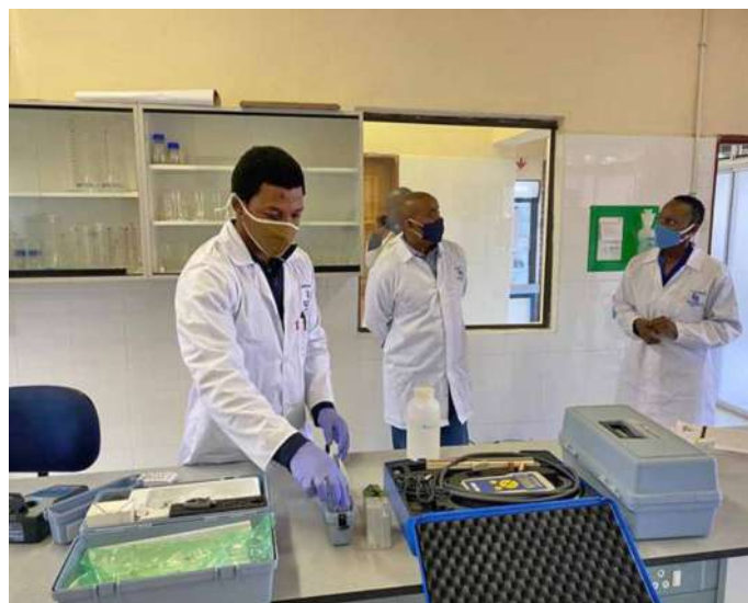
The Lab technician running a Total Solids test whilst the Environmental Officer explains the Physico-chem processes.
